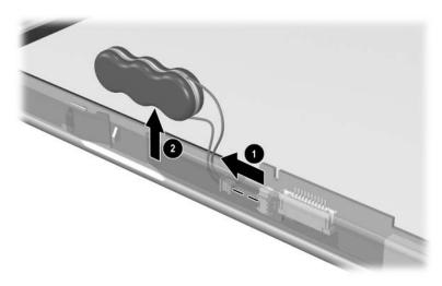
Removing the Bridge Battery
